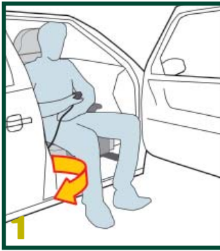
1 Using the pendant, the Turny Orbit Seat rotates out automatically...
